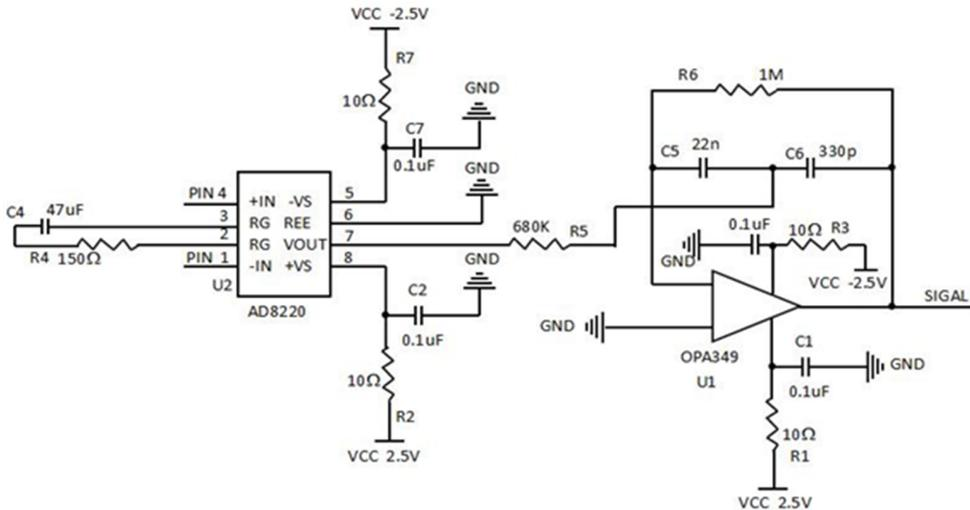
Fig. 1. Circuit diagram of enlargement and filtering
