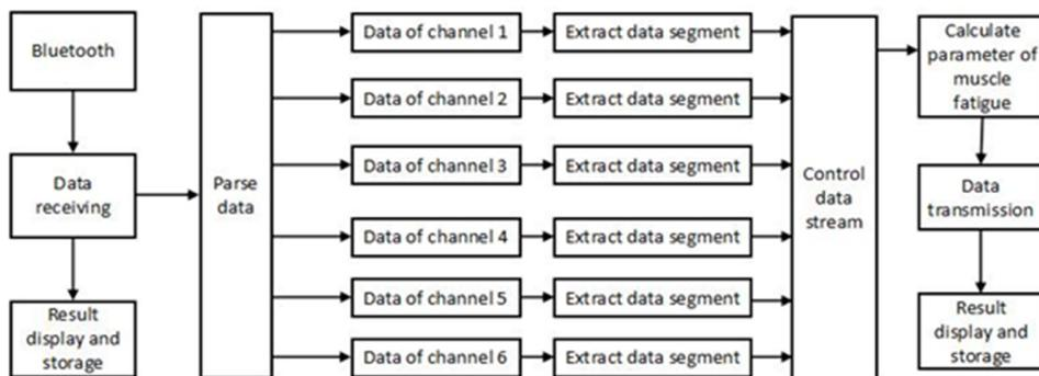
Fig. 4. Software framework of data processing module
